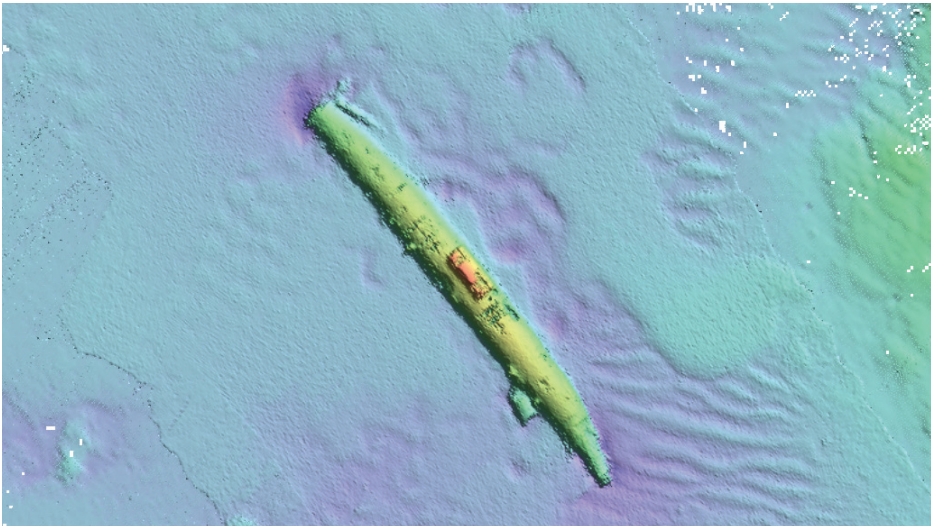
Multibeam image of the wreck of the German UC-42 submarine, lying on the sea-bed off the coast of Co. Cork. This is one of many such images produced by the INFOMAR project, which is mapping the sea-bed around the coast of Ireland and it highlights the benefits of collaborations between agencies (Image courtesy of INFOMAR/Geological Survey Ireland/Marine Institute).
